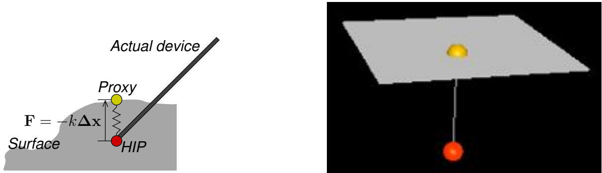
(a) When the haptic device penetrates the 3D object, the proxy remains on the surface and a spring force is returned to the user.
