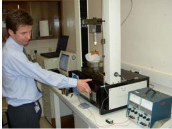
FIG. 5.6: Experimental set-up, a Chiba needle is mounted and driven into the tissue at 500 mm per minute. Image courtesy of Dr Derek A. Gould at Radiology Department, Royal Liverpool Trust.
