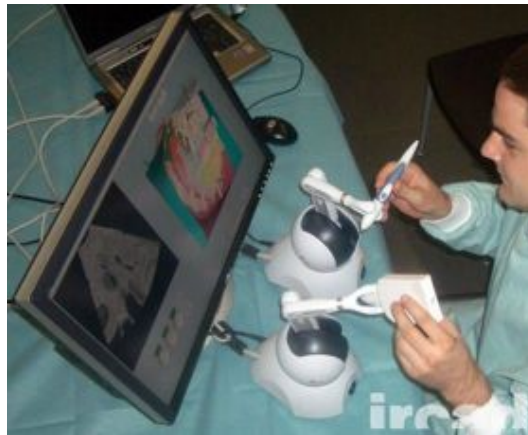
FIG. 3.37: HORUS, the US guided needle puncture simulator developed IRCAD, France. Source: Reproduced from http://www.ircad.fr/virtual_reality/horus.php?lng=en .
