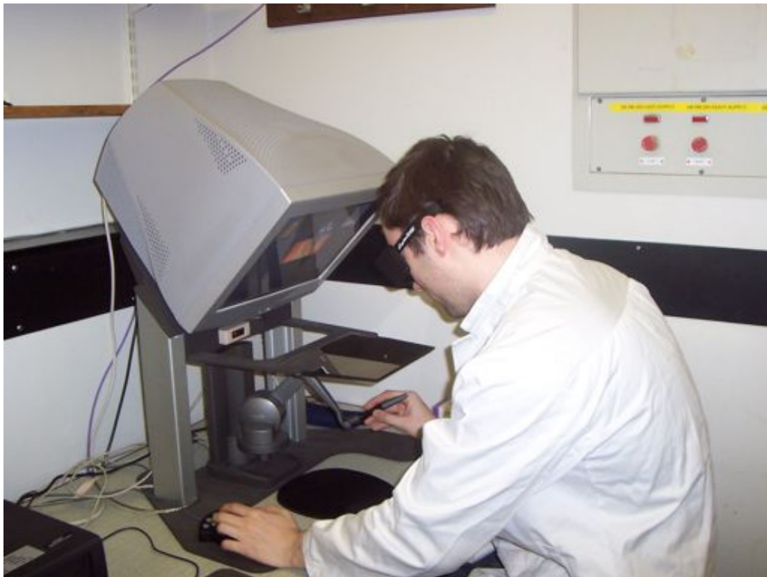
FIG. 6.11: The early VE platform presented in [265]. It makes use of an immersive virtual environment with stereoscopy, which enables the co-location of 3D graphical models with a haptic joystick.
