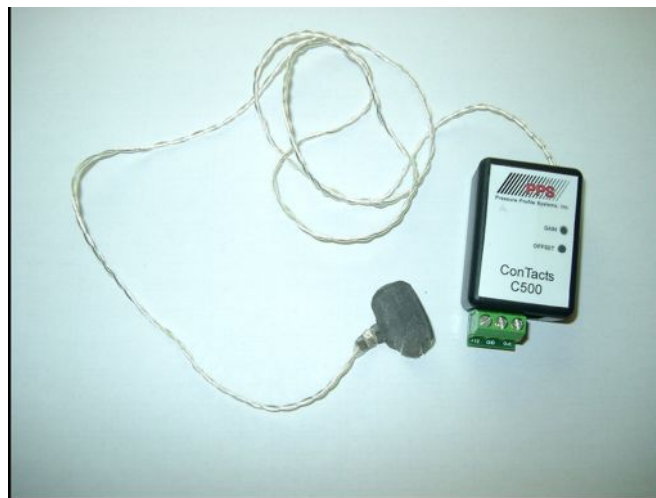
FIG. 5.4: Capacitance sensor with conditioning unit.
