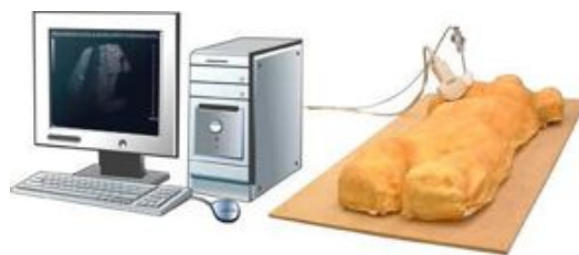
FIG. 3.38: US guided needle puncture simulator developed at Leeds University, UK. Source: Reproduced from [284].
